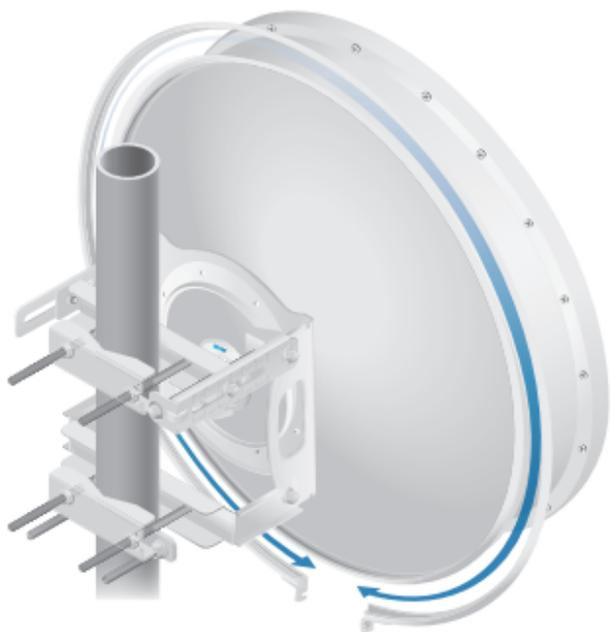
4. Secure the band clamp by tightening the screw.
