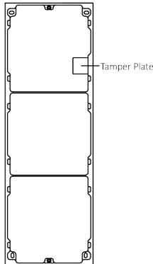
**Figure 3-32 Mounting Frame**
