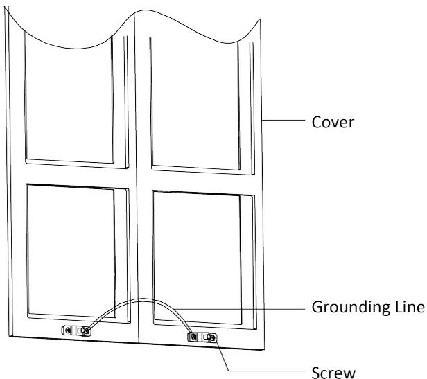
**Figure 3-62 Connect the Grounding Line to the Cover**
