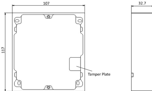
**Figure 3-2 Mounting Frame**
