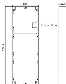
**Figure 3-44 Mounting Frame**
