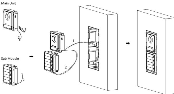
**Figure 3-27 Connect Cables and Insert the Modules**
