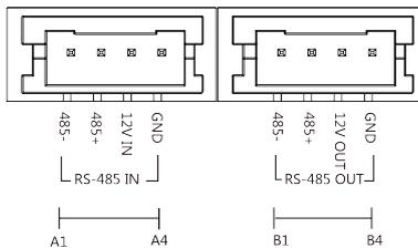
Figure 2-3 Sub Module Terminal (Except Touch-Display Module)
