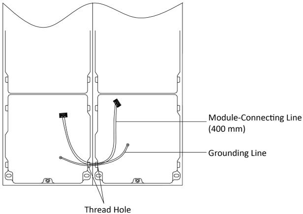
**Figure 3-46 Place the Grounding Line and Module-Connecting Line**
