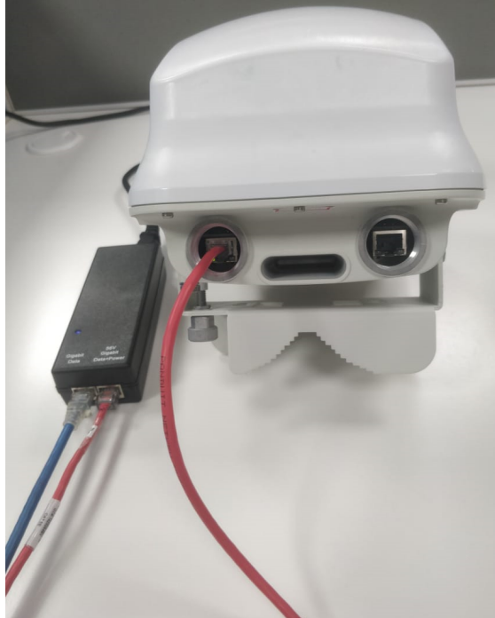
Figure 29: Connecting the V2000 power injector
