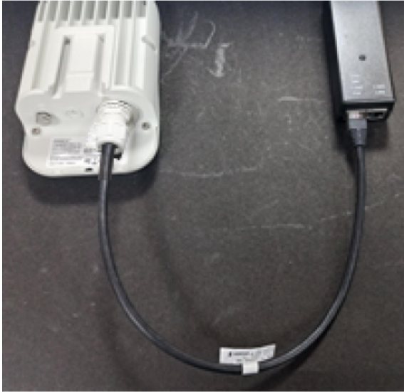
Figure 28: Connecting the V1000 Power injector
