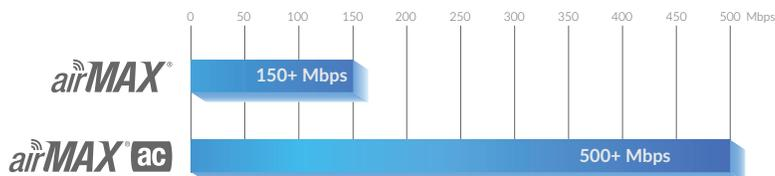
\* Up to 330+ Mbps (maximum 40 MHz channel width) for the R5AC-PTMP.
