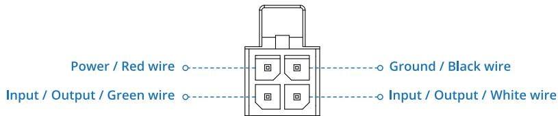
**I/O (PIN 3 and 4):** Configurable digital Input/Output pins. Open collector output, max output 30 V, 300 mA or Digital input where 0-6 V detected as logic low and 8-30 V – logic high.
