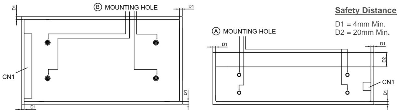
**Fig. 3 Mounting Hole Locations and the Safety Distance**
