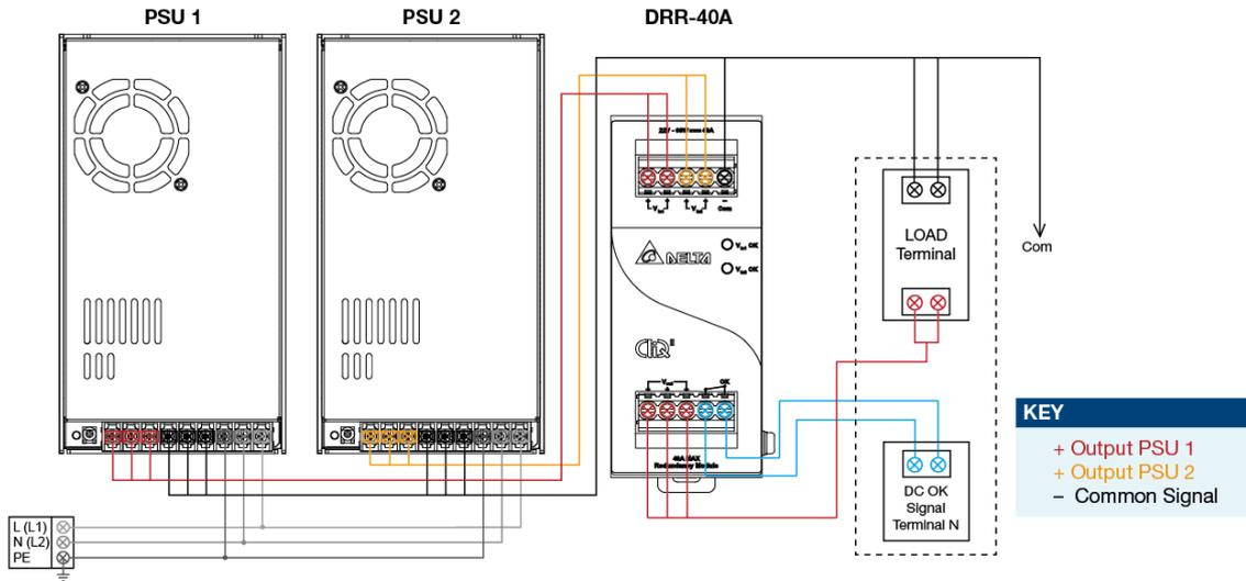
Fig. 5 Redundancy / Parallel Operation Connection Diagram
