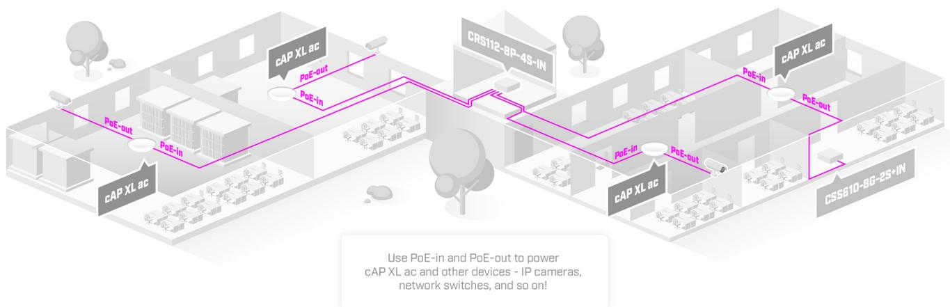
The dual-band, dual-chain 2.4 and 5 GHz wireless radio provides a strong coverage in 360 degrees around it, so you don't have to worry about the placement of the device so much. Putting it on the ceiling eliminates many signal absorption problems, such as the signal being blocked by large TV sets, metal cubicle walls in open space offices, etc.
