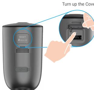
If the camera is out of battery, connect it to power outlet with the power adapter for charging (5V 2A).
