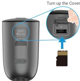
**i** After installing the Micro SD card, you should initialize the card in the EZVIZ app before using it.
