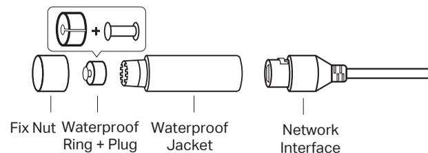
1. Insert the waterproof plug into the waterproof ring, then insert them into the waterproof jacket.
