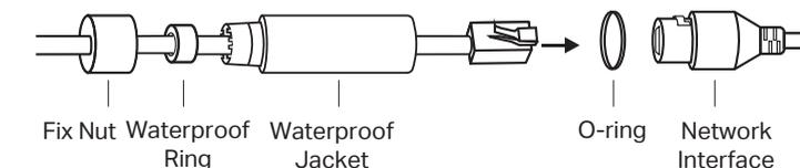
1. Route the network cable through the following components in order: fix nut, waterproof ring, and then the waterproof jacket.
