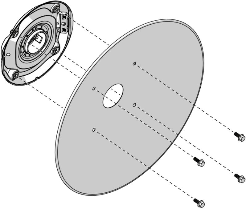
Use 10 mm Ratchet Wrench when assembling the antenna.
