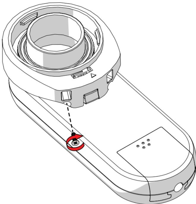
Use Phillips Screwdriver when assembling the adaptor.
