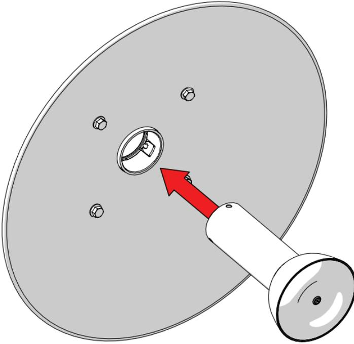
Keep twisting the Subreflector in either direction until the spring latch is engaged.
