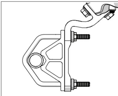
Correct orientation of the Large Pole Mount bracket is shown below,
