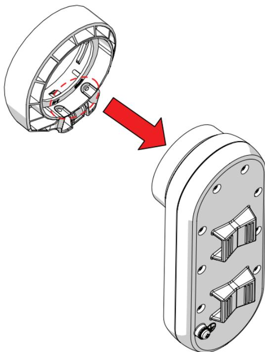
Dual Slant polarization setup
