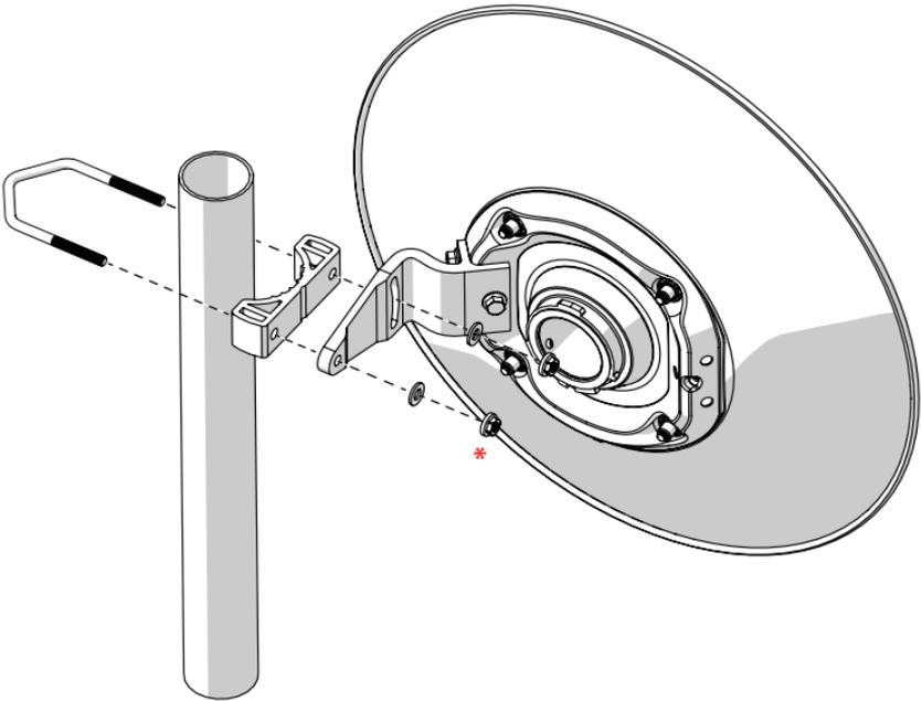
\* Optional: Surface treated M6 Nuts protect the bracket from galling.
