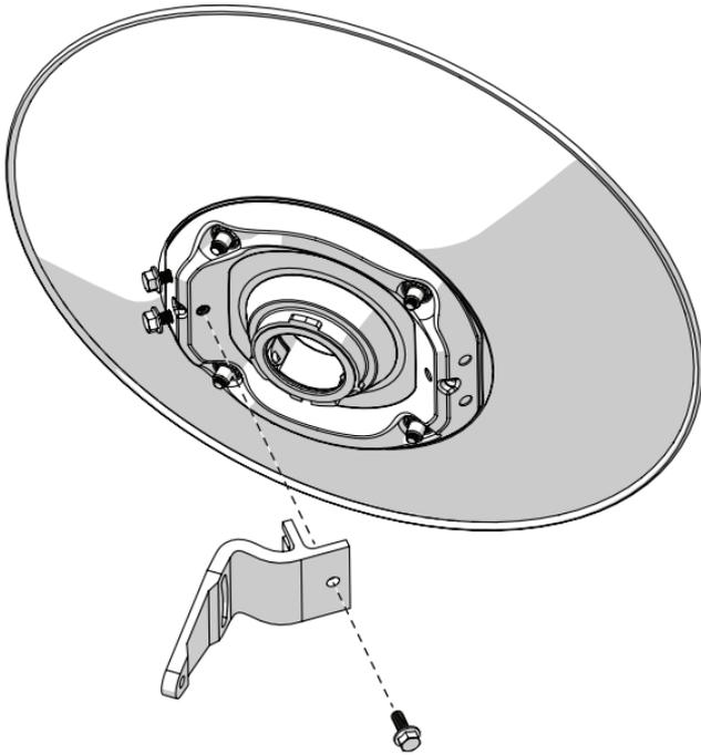
Use 10 mm Ratchet Wrench when assembling the antenna.
