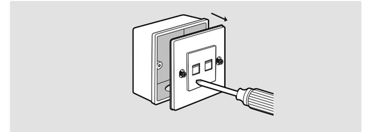
2. Detach the faceplate of the EAP with a screwdriver.
