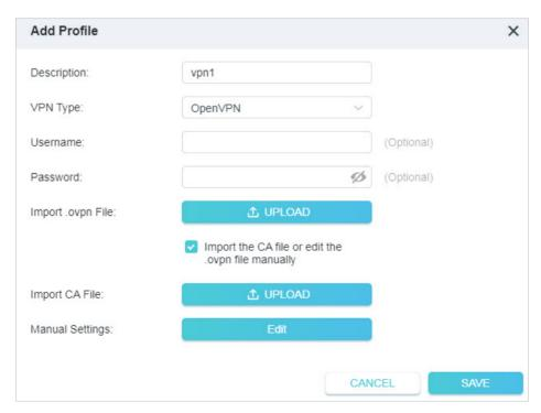
Note: You can also check the box of Import the CA file or edit the . ovpn file manually, then upload the CA file or manually configure the settings.
