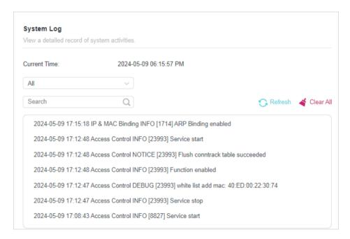
4. In the Save Log section, click SAVE TO LOCAL to save the system logs to a local disk.
