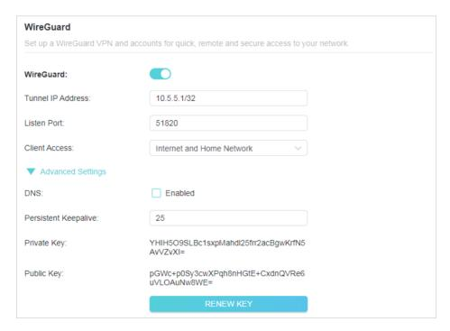
3. Set the Tunnel IP Address and Listen Port. Do NOT change it unless necessary.
