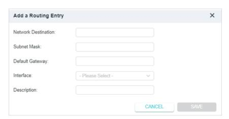
Network Destination: The destination IP address that you want to assign to a static route. This IP address cannot be on the same subnet with the WAN IP or LAN IP of Router A. In the example, the IP address of the company network is the destination IP address, so here enter 172.30.30.1.
