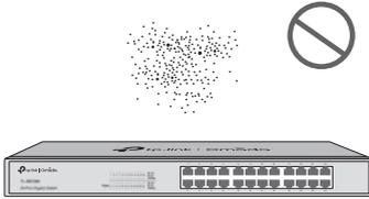
The dust accumulated on the switch can be absorbed by static electricity and result in poor contact of metal contact points. Some measures have been taken for the device to prevent static electricity, but too strong static electricity can cause deadly damage to the electronic elements on the internal circuit board. To avoid the effect of static electricity on the operation of the switch, attach much importance to the following items:
